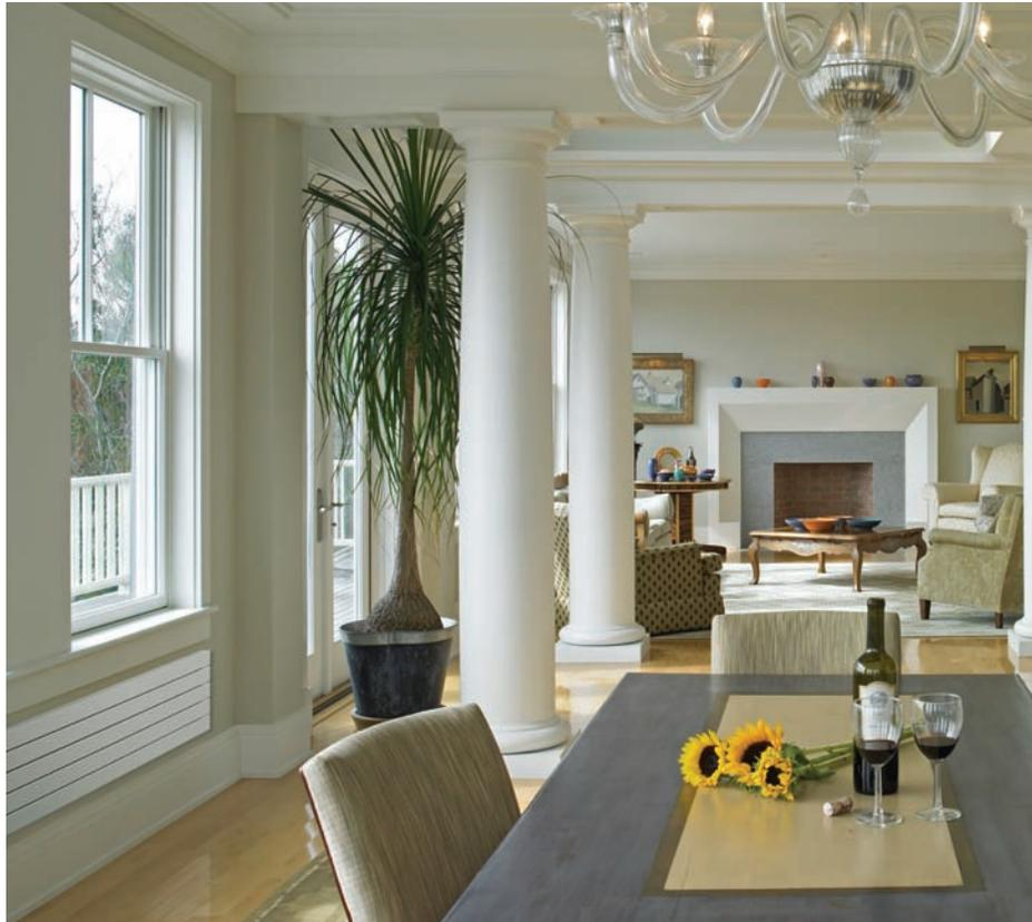
**Runtal's Wall Panel style radiators** are ideal for placement under windows or on walls where floor space is at a premium. When placed under windows, wall panels help eliminate cold spots and drafts while allowing curtains to hang to the floor. Wall panel radiators are available in a variety of heights and widths to suit most any need.
