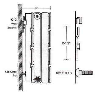
${\bf R}$  clip - Mount to the Cutouts on the RF Radiator at the K12 Positions
